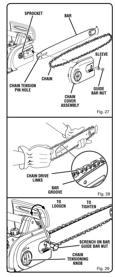
Reinstall the chain cover assembly, bushing and guide bar nut. Tighten the guide bar nut finger tight only. The bar must be free to move for tension adjustment.
